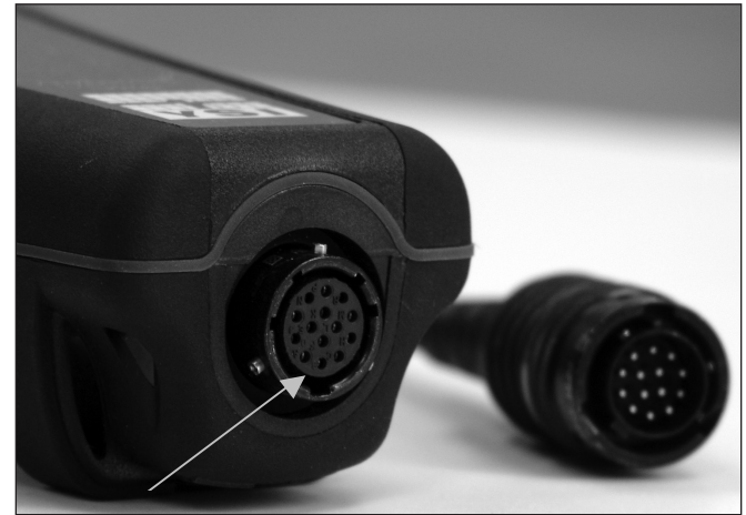
Figure 4, Note the keyed connector.
